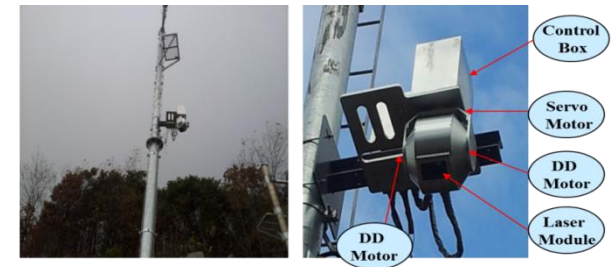
Fig. 3. The appearance of the developed laser scanner based on robot technique
