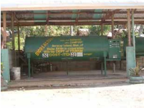
Photo: Bioreactor to prepare compost from biodegradable waste
