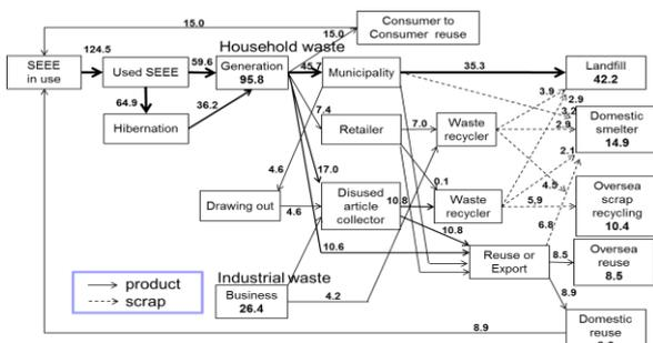
Fig. 1 Material flow of used small electrical and electronic appliances (except personal computers, mobile phones or car items)
