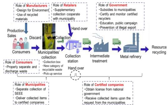
Fig.2 Role of stakeholders under the recycling system of used small electrical and electronic appliances
