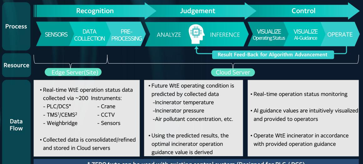
\* ZERO4wte can be used with existing control system (Designed for PLC / DCS)
